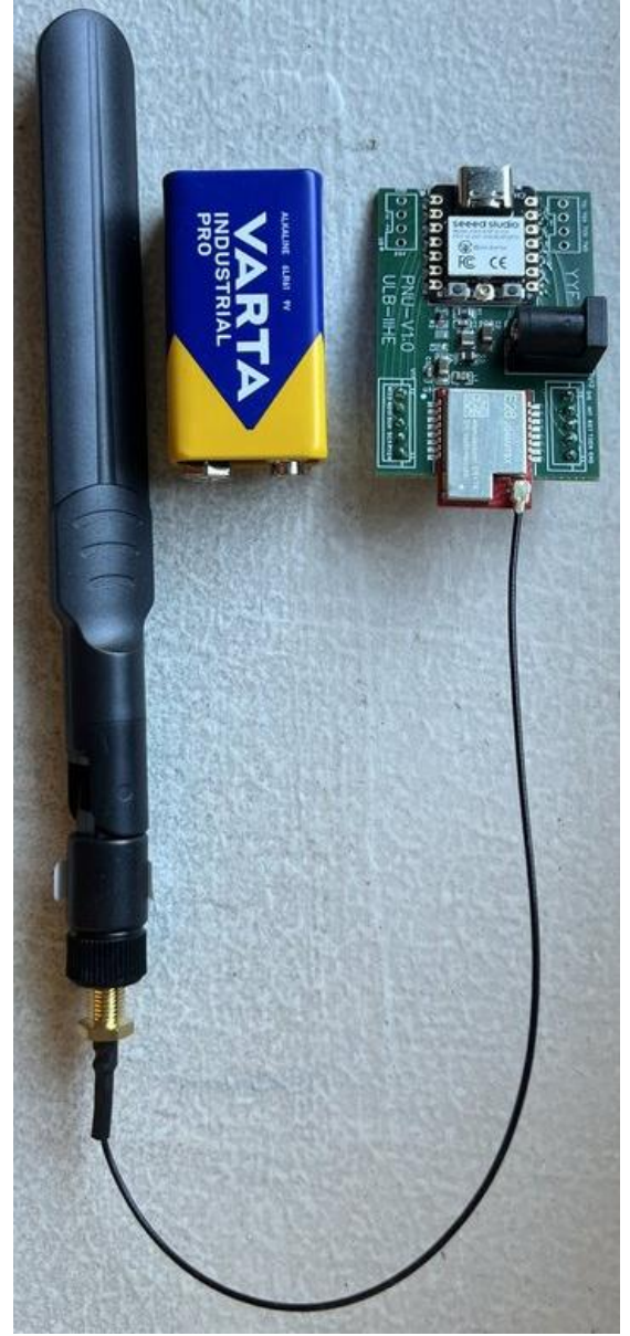
Fig. 4. PNU V1.0 hardware prototype (marked “PNU-V1.0 ULB-IIHE”). The custom PCB integrates the Ebyte E28 module and Seesee Studio XIAO ESP32, powered by a 9 V VARTA industrial battery through a regulated power rail. An external 2.4 GHz SMA antenna is attached.
